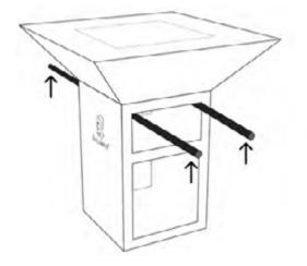
c) Adjust the position of the hearth using a level. This is especially important in order to avoid fat and juice from the grilled food overflowing to one side. Adjustable screw feet can also be used (attached). Once the grill is level, you can anchor it to the underlying pedestal (attached). The original anchor kit comes with a lock, but VULCANUS® can be moved at any time. This solution is suitable, for example, for public places and for security purposes.
